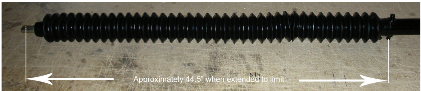
Fig. 5 Extended Limit should be adjusted so a completely extended actuator measures approx. 44-1/2" center to center. This dimension does not need to be especially precise.
